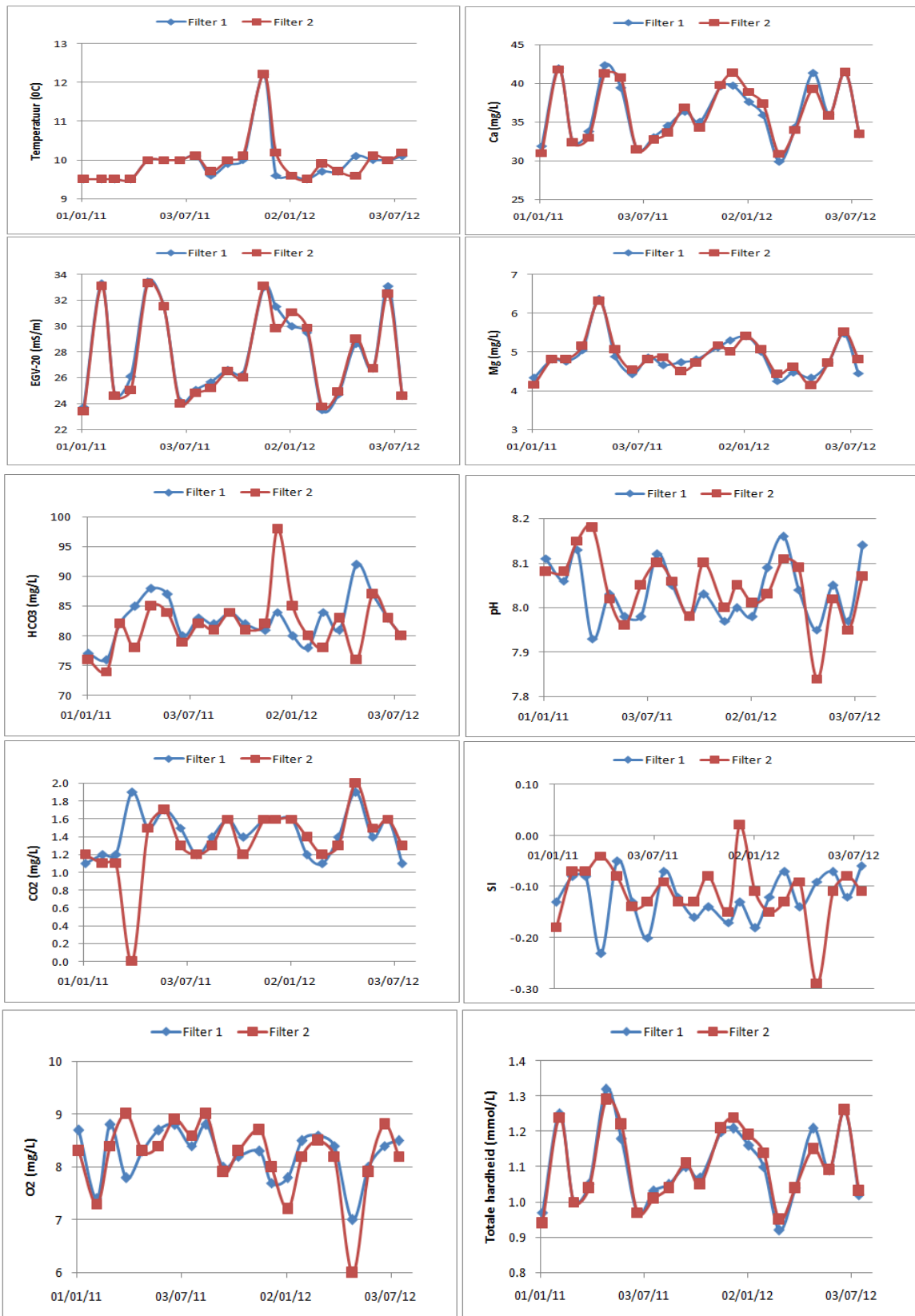
Figure 66: Measurements of post-filtrated effluent at Honderloo
