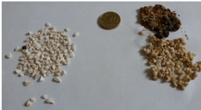
Figure 37: The relative sizes of the top layer filtering marble grains and feeding grains in the reference of a 10 cent Euro coin
