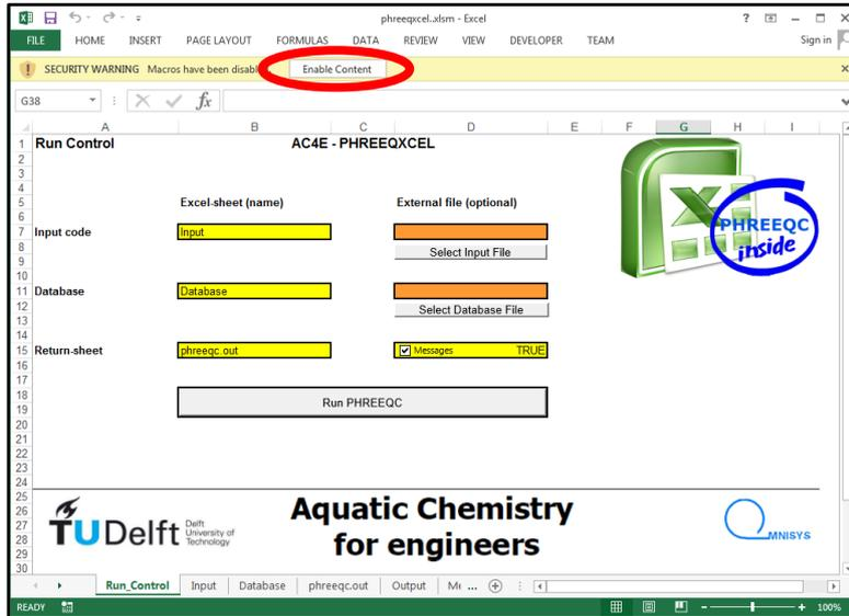
On opening a PhreeqXcel application the PHREEQC-code on sheet Input is executed, in 'silent' server-mode, as defined in the VBA-sub 'Workbook\_Open'. This run includes the initial loading of the COM-module.
