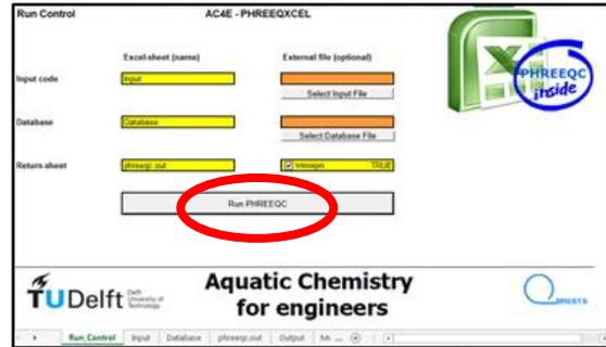
Starting the PhreeqXcel application runs the simulations defined in the user input code on sheet 'Input' using the PHREEQC database on sheet 'Database'. The results are presented on the sheets 'Output' and 'phreeq.out'.
